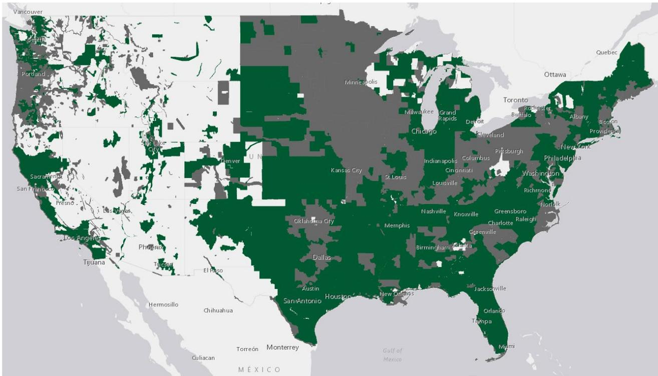
**Figure 1.** Map of lidar coverage for the contiguous United States, March 2019. Gray represents publicly available lidar of any quality level and collection date; green represents lidar satisfying USGS 3DEP baseline specifications. 3DEP-quality lidar data is available for approximately 53% of the nation. Montana lidar coverage of any quality is approximately 30%. (Figure from online web application, Seasketch: U.S. Federal Mapping Coordination).
